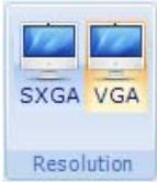
The SDP 860 USB Viewer program supports 2 output resolutions: SXGA and VGA. (SXGA runs at 15 frames per second while VGA does at 30 frames.)
